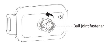
• Put the clip through the ball joint fastener, and assemble the clip ④ on the wireless car charger.
