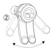
• Remove the ball joint fastener ③ from wireless car charger by rotating it counterclockwise.
