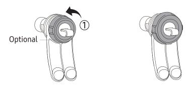
• Set the support frame ② with proper angle to suit for your car's air vent.
