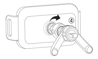
• Rotate the control knob ⑤ to adjust the length of metal hook, so that the wireless car charger which has been assembled already can be locked on the air vent of car⑥, then connect the USB Type C cable to the port.
